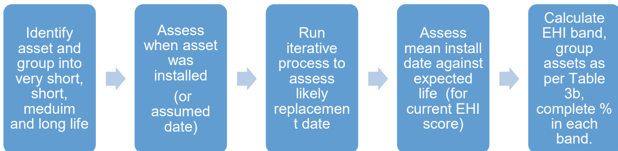
Figure 3 - Process to forecast the 'Basic' EHI score for March 2033 and March 2051 (using level 1 model)
